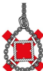
If chains are mounted around a load (e.g. support arms), the diameter needs to be a minimum 3 x the chain pitch (inside chain link length); if using a smaller diameter, the load capacity must also be reduced by 50 %.
