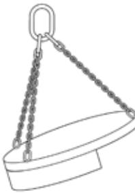
Figure 15: All the load is carried by two chain legs
