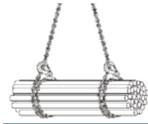
Figure 11: Wrap and choke hitch
